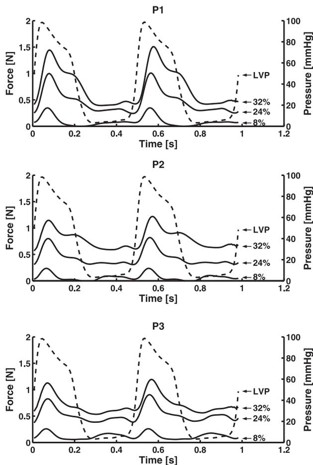
**FIGURE 2.** Representative traction suture force curves throughout the cardiac cycle. *Broken line*, left ventricular pressure (LVP). *Solid lines*, force curves at downsizing percentages of 32%, 24%, and 8%, corresponding to approximately 16 mm, 12 mm, and 4 mm external suture tightening, respectively.
