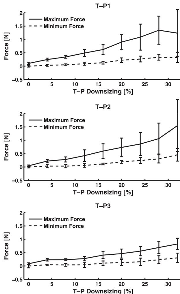
**FIGURE 3.** Absolute maximum and minimum force magnitudes as a function of incremental annular downsizing (%; mean  $\pm$  one standard deviation). The values are average measurements of the downsizing and force measurements between the right trigone (T) and the posterior annulus segments (P1, P2, and P3).
